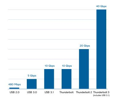
A single cable now provides four times the data and twice the video bandwidth of any other cable, while also supplying power
